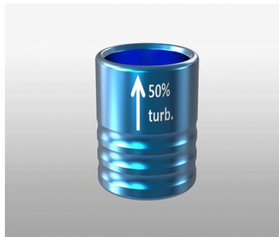
Reference normal for verification - backscatter measurement
